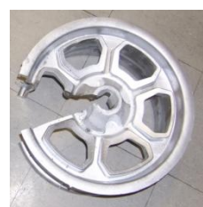
CAST WHEELS ARE FETTLED IN FOUNDRY TO REMOVE SPRU & FLASH FROM CASTING
