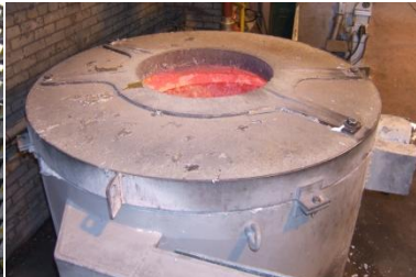
PRIMARY ALUMINIUM IS MELTED IN THE FURNACE @ 900 DEGREES C
