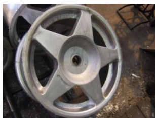
CAST WHEELS ARE FETTLED IN FOUNDRY TO REMOVE SPRU & FLASH FROM CASTING
