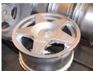
CAST WHEELS ARE FETTLED IN FOUNDRY TO REMOVE SPRU & FLASH FROM CASTING
