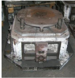
COMPLETE DIE TOP CORE, BOTTOM CORE & DIE SIDES ARE ASSEMBLED READY TO GO ON CASTING MACHINE
