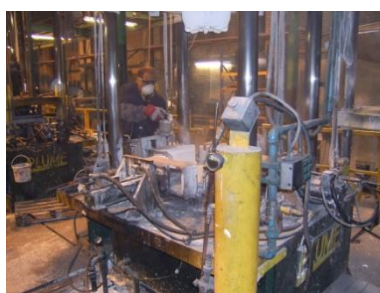
BATCHES OF 60>250 WHEELS ARE LOW PRESSURE CAST IN SPECIALIST PLUME MACHINES
